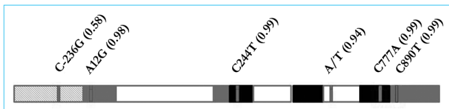
Figure 3. Representative scheme of the AANAT gene and the polymorphism that we have found. The hatched area represents the gene promoter region, the introns are represented by the white areas. The grey rectangles are the exons non-coding region and black represents the coding regions. Grey vertical bars indicate the polymorphisms positions. The numbers between parentheses are the allele frequencies found in this study
